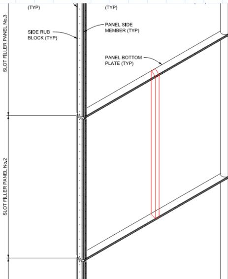
This stiffener will be the same size (if not larger) than the two side HSS members. Therefore no specific checks are required for this member
