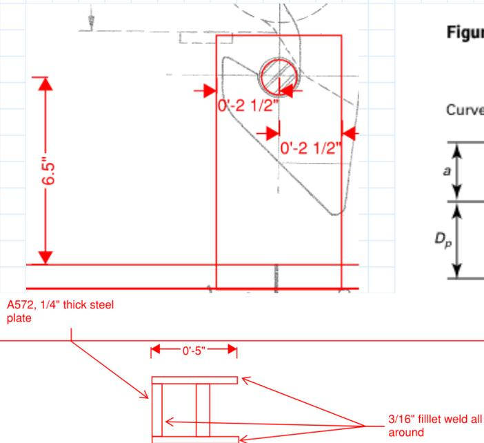
Figure C-3.3.1-1 Pin-Connected Plate Notation
