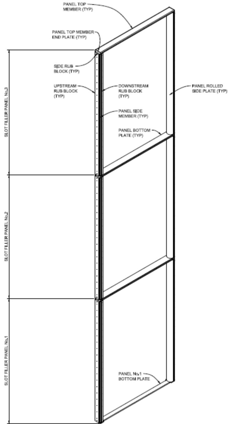
A total of 3 slots will need frame fillers at the North and South entrances (wider span openings) and 6 total slots will need them at the East and West entrances (shorter span openings).
