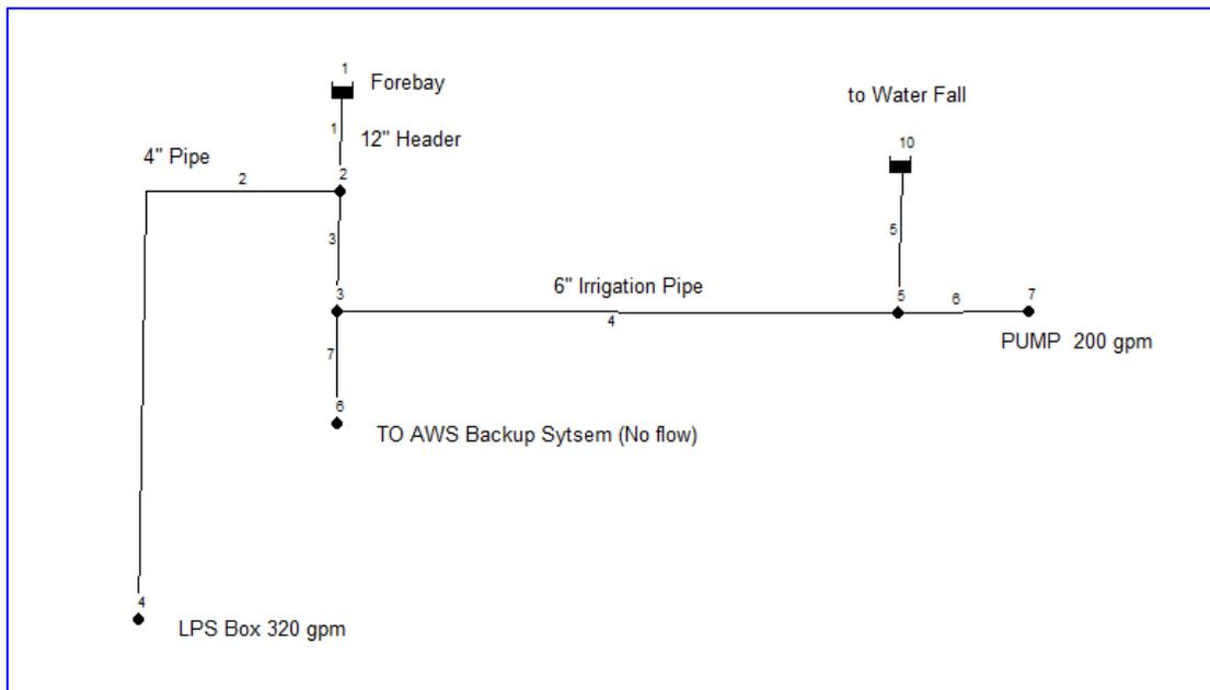
According to the EPANet pipe network model, the LPS system flow requirements have near non-detectable effects on the irrigation system and vice versa. The EPANet results are provided in Appendix B, Item B-2.
