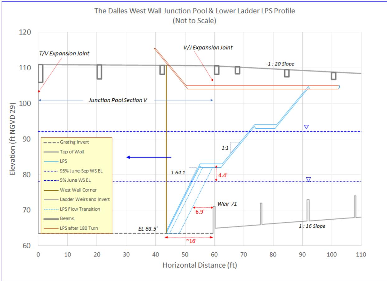
The proximity of the west-wall LPS to weir 71 necessitates a flow deflection transition on the upstream side of the LPS to minimize the flow disruption in the vicinity of the weir crest (see Figure 3-15 for proposed plan view of deflector transition). Bonneville Second Powerhouse Adult Fish Facility (AFF) used a similar approach with a closer proximity (~ 3.4 feet) to the crest of the bottom weir in the ladder exiting the AFF laboratory.
