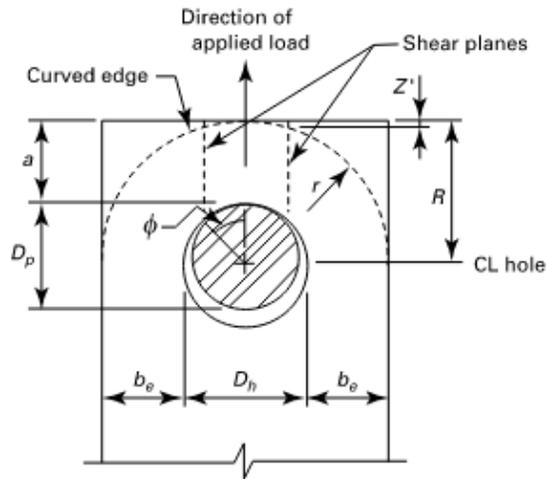
Static strength of the plates: ASME BTH EQ, 3-45
