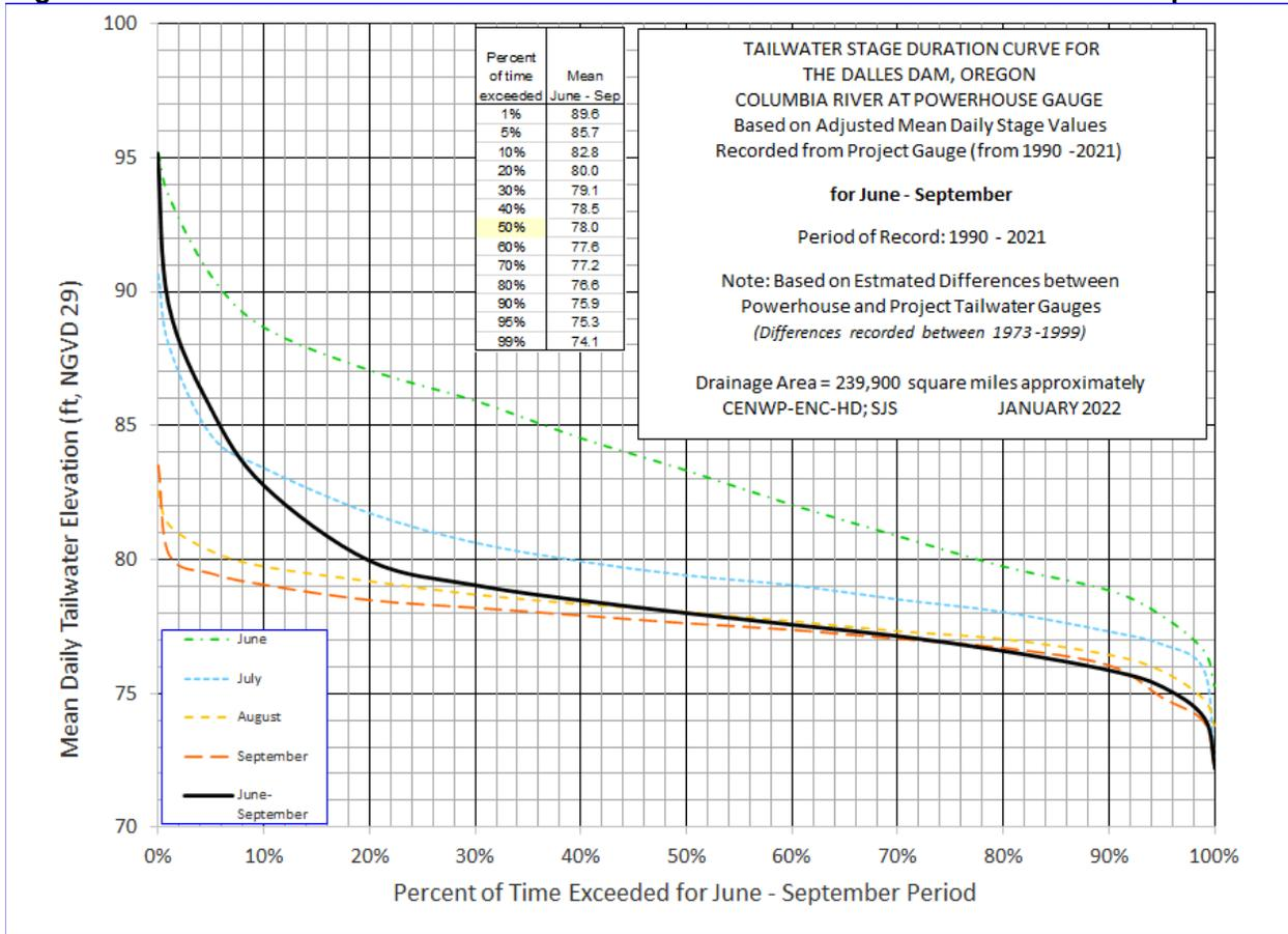
The lowest rest box needs to be located above the maximum expected level expected in the Junction pool. The pool water levels will be about 2.5 feet higher than the tailwater elevation.
